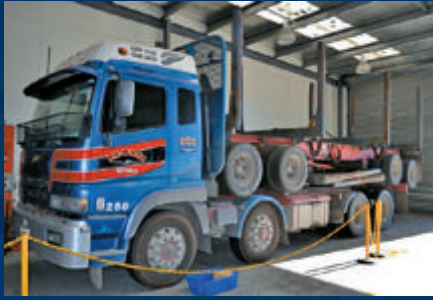
2011 Mitsubishi Fuso Shogun F5430S9 8x4 Logging Truck & Trailer , 430HP, Eaton 18 Speed, 6-Rod suspension, GVM: 30,800kg GCM:52,000kg Tare: 10,620kg, comes with 4-axle Koromiko Logging gear
