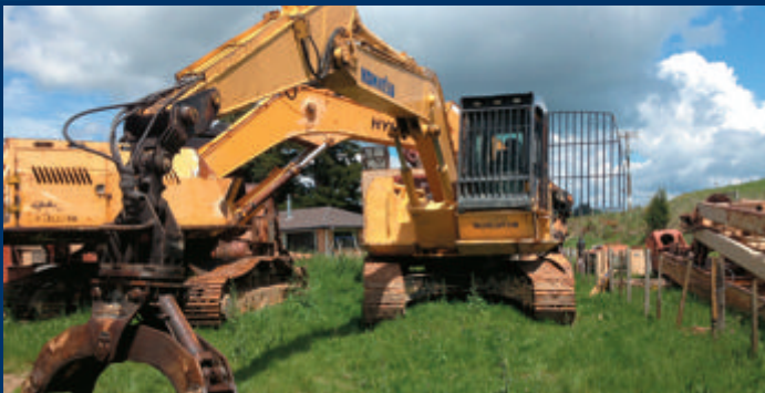
X1 Komatsu 220LC high & wide with ops, cops and fops fitted with Ensign 20T 1500 rotator grapple, showing 13,445 hrs on the meter, tracks done in 2013.
